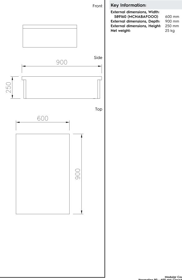
Modular Cooking Range Line thermaline 90 - 600 mm Closed Work top, 1 Side
